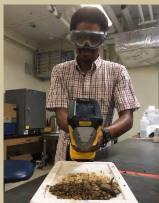
Dr. Richardson using portable X-ray Fluorescence (pXRF).
